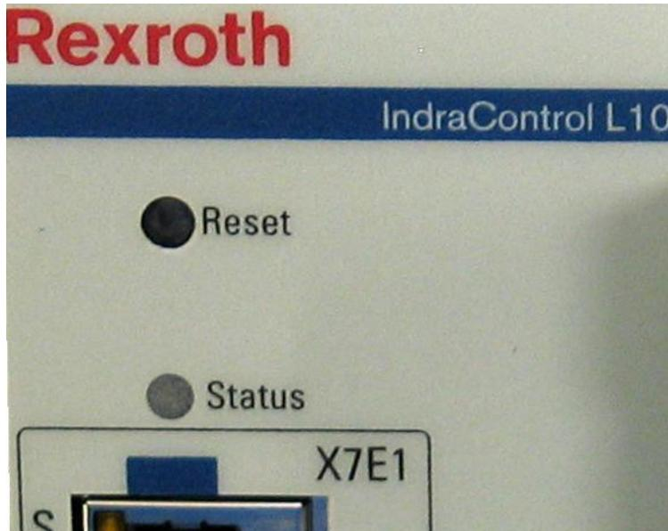
The **reset button** can only be pressed using a tool, for instance with the tip of a pencil.
